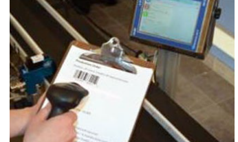
Job data can be sent to the printer via a hand-held scanner
